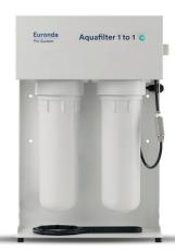
Device for the production of deionised water for autoclaves, in accordance with EN 13060 (< 15  $\mu$ S/cm). Only one Euronda Pro System autoclave can be supplied. It deionises on average 1 litre of water per minute. It can be equipped with automatic shut-off device. It can be placed directly on the worktop or inside a cabinet, as well as mounted to a wall. Included in the initial equipment are two ion exchange resins.
